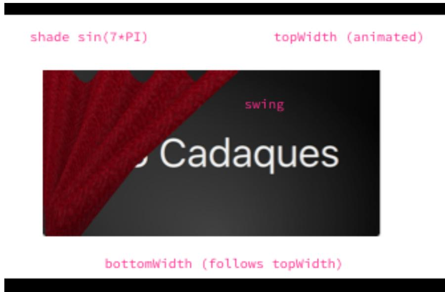
The waved shades of the curtain are computed through a sin curve with 7 up/downs ( $7*PI=21.99\dots$ ) on the width of the curtain. The other important part is the swing. The *topWidth* of the curtain is animated when the curtain is opened or closed. The *bottomWidth* follows the *topWidth* with a *SpringAnimation*. By this we create the effect of the swinging bottom part of the curtain. The calculated *swing* provides the strength of this swing interpolated over the y-component of the vertexes.
